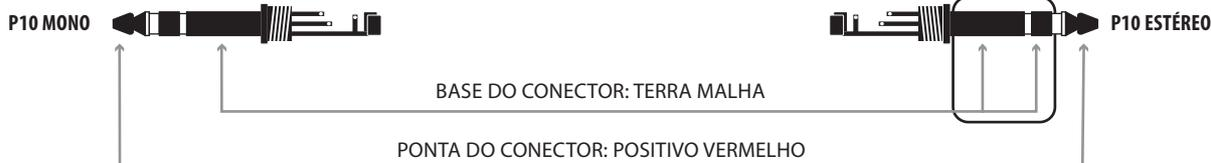
NO CONECTOR DO PROCESSADOR VOCÊ DEVE UNIR A BASE AO CENTRO OU UTILIZAR UM CONECTOR MONO.
